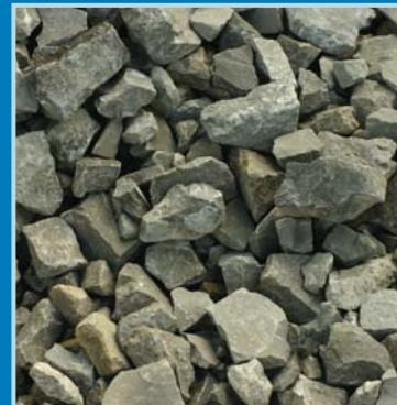
Porous pavements. Uncompacted gravel, crushed stone, and open paving blocks reduce or eliminate runoff and allow rainwater to filter into the ground.
